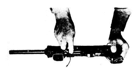
Figure 8. Remove the magazine catch assembly by rotating it twoard the right side of the receiver.
