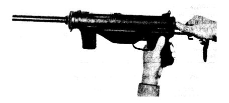
Figure 5. Press in on stock catch on the left side of the pistol grip, and remove the stock by pulling it directly to the rear.
