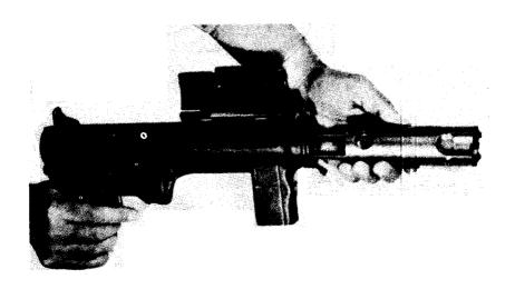
Figure 11. Open the cover, and withdraw the bolt and guide rod group from the receiver.
