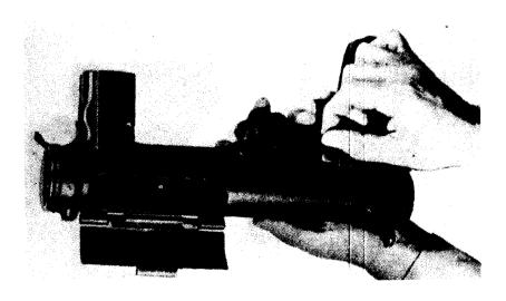
Figure 13. Remove the trigger pin.
