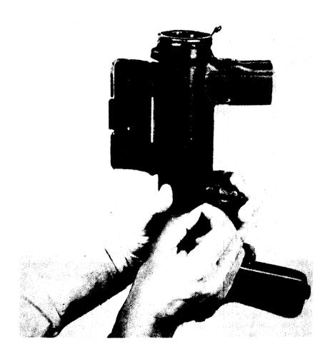
Figure 17. Grasp the receiver, with the little finger on the trigger and the first finger against the sear. Press down on the trigger, and at the same time manipulate the sear until the sear pin hole in the sear is alined with the hole in the receiver. Replace the sear pin.
