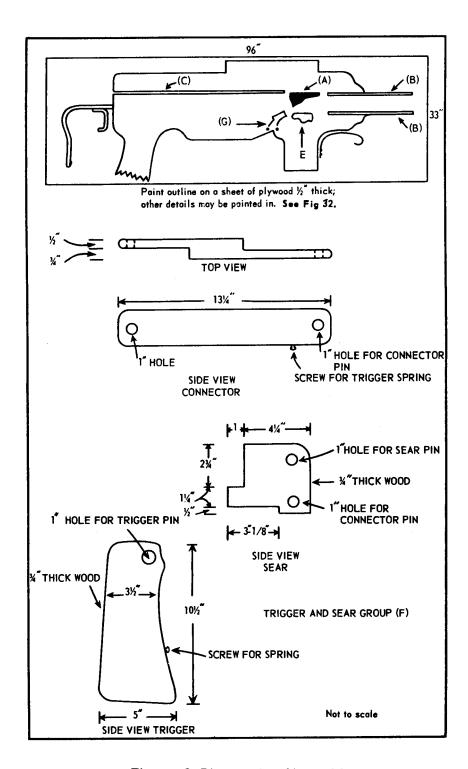
Figure 331. Diagram of working model.
