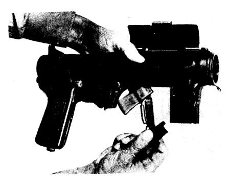
Figure 14. Withdraw the trigger and sear group from the receiver. Be careful not to drop the connector pin. This completes field disassembly.
